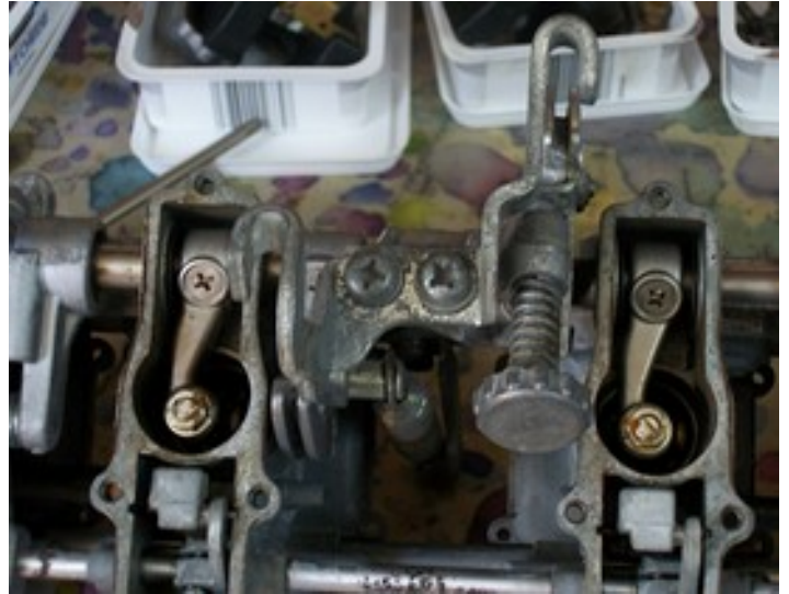
Throttle cables mount plate
