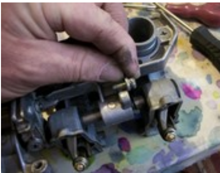
Throttle shaft stopper plate screw
