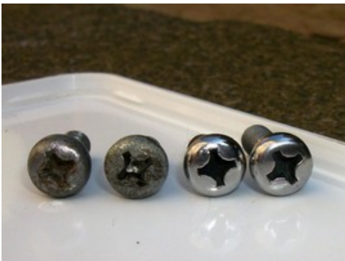
Carb to head screws before and after plating
