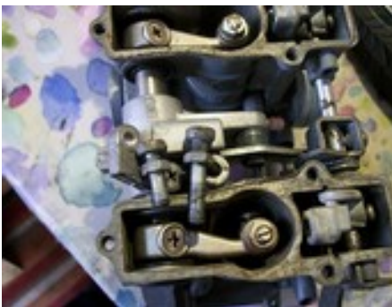
Fast idle and throttle stop screws
