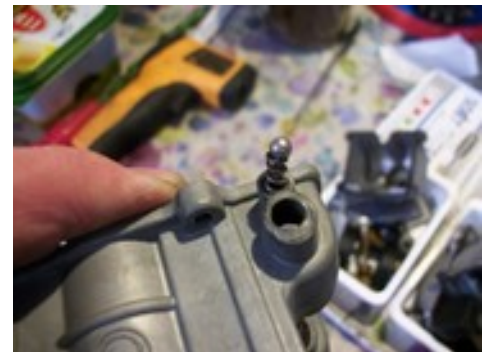
Choke lever ball bearing and spring
