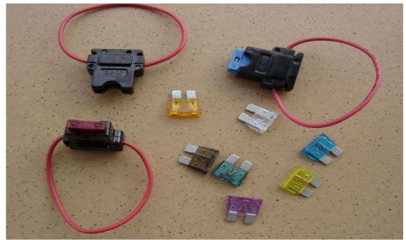
Here are typical blade fuse holders and fuses, each colour represents a value. The red lead just gets cut and joined to the wires being run.
