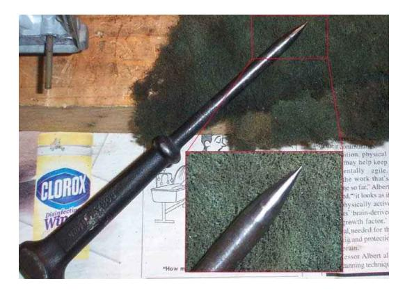
Put the awl down through the slide opening as shown below. Be careful not to scratch the walls of the slide canal. Use very little force, get the awl right on the top of the tip. Use just a small bit of pressure and push straight, do not twist or wiggle. If it doesn't pop right out, reposition and try again. It will pop out. Put your finger over the end as shown to catch it if you want.
