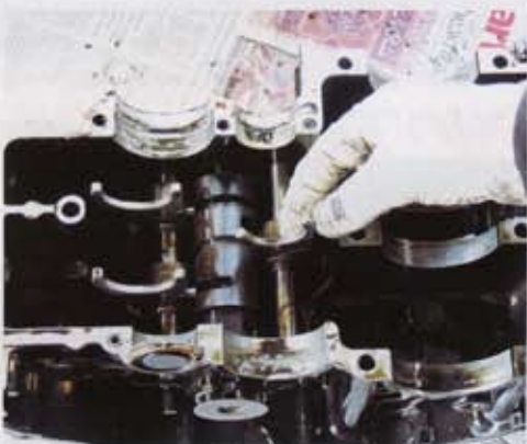
19: The lower crankcase half carries the gear selector drum and forks. These are now simple to remove, but I'm always careful to mark which location the selector forks have come from.
