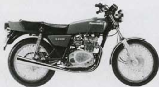
Z250B was budget version with 2LS brake and spoked wheels.
