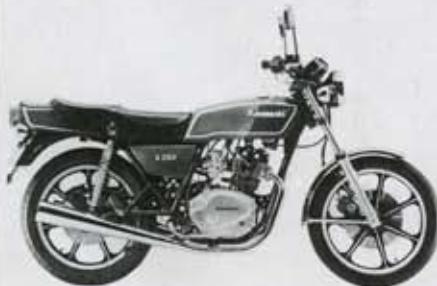
1979 Z250A1 developed 27bhp @ 10,000rpm.
