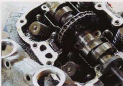
13: The cam cover lifts free once all the bolts have been removed, revealing the camshaft and its drive chain. The rockers are captive on the underside of the cam cover – I'll take a look at them later – but the cam lobes on the right-hand side look a bit battered. Note the top of the rear tensioner blade behind the camchain, and the eight domed nuts that retain the cylinder head.
