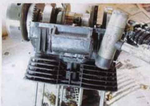
20: I've been lucky here. A bit of gentle persuasion has shifted the barrels off the crankcase mouth and I can proceed to tap them down the studs with a rubber mallet to release the pistons from the bores. It's easy to damage a fin this way so carefully choose where you apply force.
