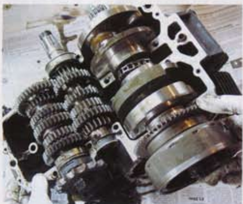
18: Note the camchain sitting loosely on the crank sprocket. Behind the crank is the input shaft, and behind that the output shaft. Six cogs on each shaft confirm this is a six-speed box.
