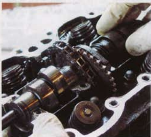
15: Now the camchain is slack I can remove the two M6 bolts that hold the camchain sprocket to the camshaft and drop it down, off its mounting, onto the side of the cam journal.
