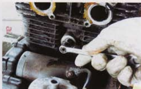
14: Before I can remove the camshaft I need to slacken off the chain. The camchain tensioner lives behind the cylinder barrel, and is a pretty substantial device – rather reminiscent in fact, of the Yamaha design fitted to the XS650. Unlike Kawasaki's bigger 400 and 750 twins the Z250/305 uses gear primary drive instead of chain, meaning the crankshaft rotates 'forwards' and the tensioner is at the back of the barrels, not the front.
