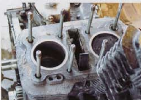
16: With the camshaft out of the way I can slacken and remove the eight cylinder head nuts, working in a diagonal sequence, then lift away the head. Now the front camchain slipper blade is revealed. The oil feed for the cam bearings travels upwards through the two rear outer stud holes – note the O-rings fitted into the gasket to prevent leaks.
