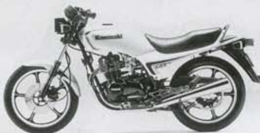
Final version of the Z250 twin had Unitrak suspension and belt drive.
