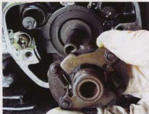
12: Behind the points plate is the auto advance unit, driven at half crank speed on the end of the camshaft. This, at least, looks to be in serviceable condition. There's an oil seal behind the unit, sandwiched between the head and the cam cover, which will be replaced on the rebuild.
