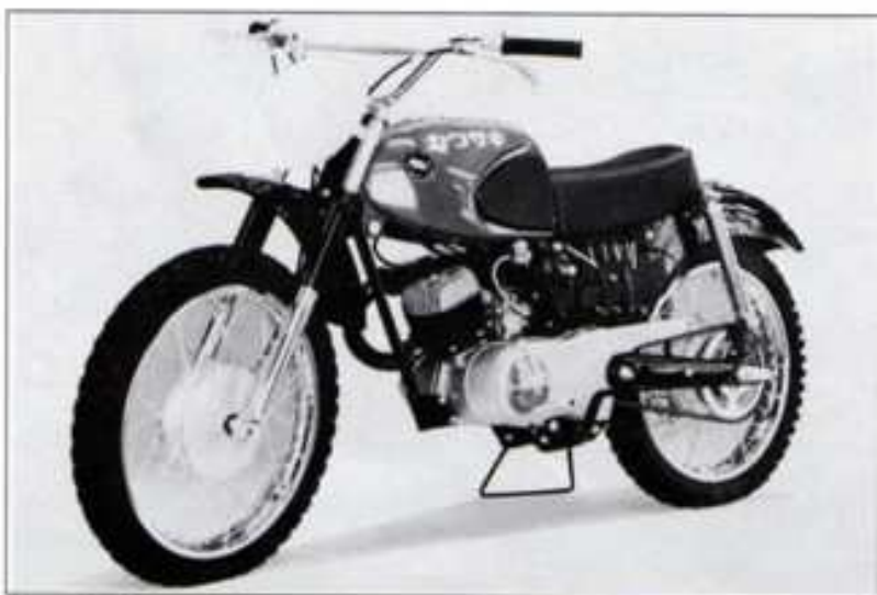
Kawasaki's first production motocrosser was the four-speed 125cc B8M of 1963. With its distinctive red fuel tank, this highly successful machine was important in establishing Kawasaki as a credible motorcycle manufacturer. (Kawasaki)
