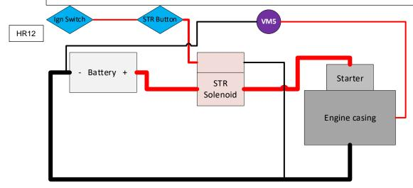
This process can be used to diagnose any resistance fault in any circuit, it looks long winded but below I have converted the above into a test plan for the starter circuit which once you have access to the solenoid, starter and battery would take approx 10 - 20 mins to accurately diagnose your starting fault (if electrical, not mechanical)
