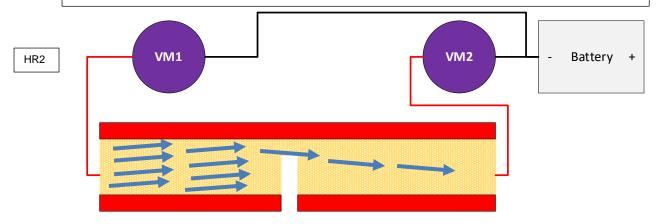
Whilst the above may seem like an extreme example the principle is relevant to any damaged or partially broken conductors.
