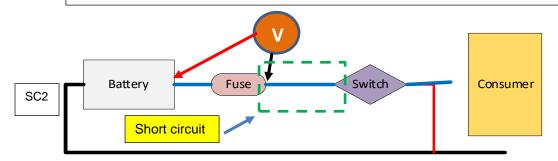
If there was not a voltage reading in the above step now operate the switch, a voltage reading now will indicate a short to ground between the switch and the consumer
