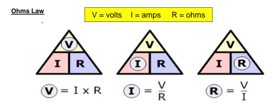
**EG:** 12v system with a 2 $\Omega$  consumer - 12v/2 $\Omega$  = 6amps
