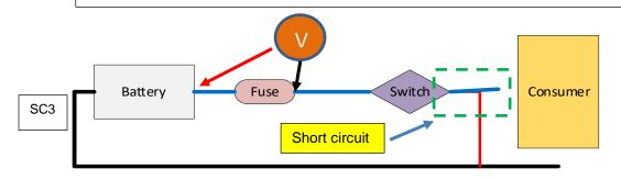
If the above test did not indicate a voltage when the switch was activated then the fault is the consumer/component itself and this should be replaced.
