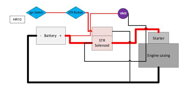
If the live at the starter main terminal was approx 0.5v or less then you should check the ground ref the below
