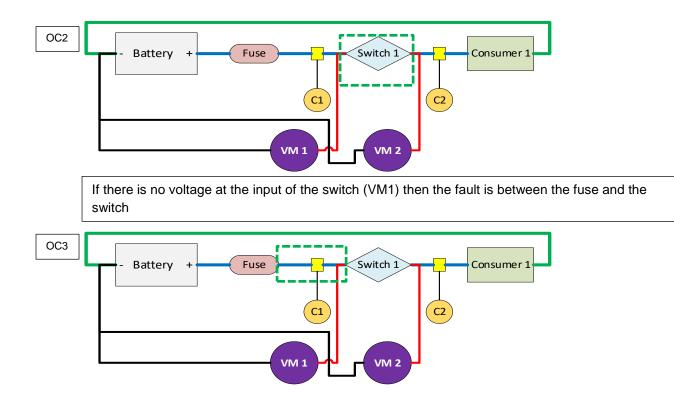
If there is voltage at the output of the switch (VM2) then the fault is between the switch and the consumer
