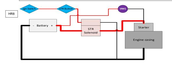
If the 1<sup>st</sup> reading was higher than approx 0.5v move the black meter lead to the output side of the solenoid and operate the starter again. A reading of approx 0.5v or less means the fault is between the solenoid and the starter (poor connection or damaged cable) if the reading is more than approx 0.5v move the black meter lead to the input side of the solenoid and operate the starter again
