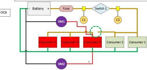
When checking wiring for breaks there are a couple of ways to locate the problem
