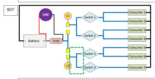
If your initial voltage reading with all the switches turned off was 0v you now need to disconnect all the consumers fed by that fuse. Now turn on and off each switch in turn until you get a reading of battery voltage
