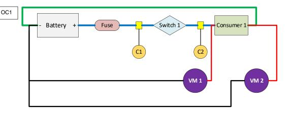
With open circuit faults the most time efficient way to diagnose is to break the circuit into sections (virtually) and to look at which points are easiest to access. If the fault is in the live side of the circuit (no voltage at the consumer) the next easiest point to check (in most cases) would be the switch.
