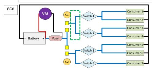
Disconnect connect C1 – If the voltage reading drops to Zero the fault is between C1 and the switches. If not disconnect C2, if the voltage now drops to 0v the fault is between C2 and the switches
