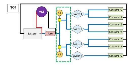
If there are any connectors between the fuse and the switches (C1 & C2) you can break it down further. Disconnect connect C1 – If the voltage reading drops to Zero the fault is between C1 and the switches
