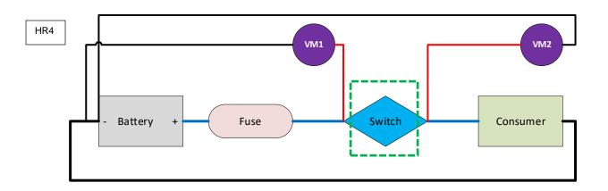
A reading of more than 0.5v less than reference voltage would indicate a resistance between the fuse and the switch (or the connections to them)
