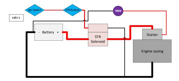
If the above reading was higher than approx 0.3v move the red meter lead to the engine casing and operate the starter. A reading of approx 0.3v or less now would suggest a build-up of dirt or corrosion between the starter body and the engine casing causing a poor ground. A reading higher than approx 0.3v would suggest a faulty ground between the engine and battery negative terminal
