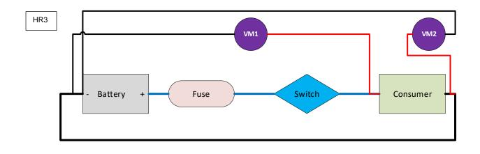
Having found that your resistance is in the live supply side the next step is to check the voltage in and out of the switch, VM1 should read approx reference voltage and VM2 should read the same approx reference voltage as VM1. A lower reading on VM2 would indicate a faulty switch (or the connections to it)
