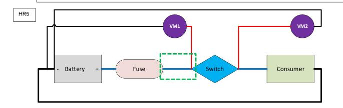
A reading within 0.5v of the reference voltage at VM2 would indicate a resistance between the Switch and the consumer (or the connections to them)
