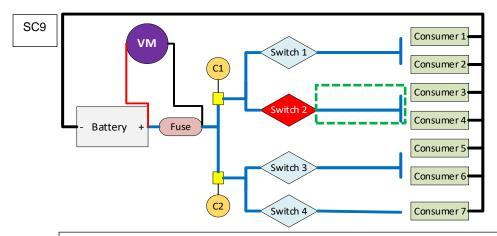
As before if none of the switches generates a battery voltage reading at the output of the fuse one of the consumers fed by that fuse is faulty.
