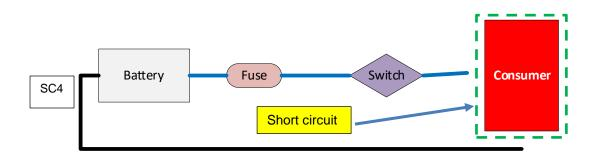
To find a fault in the wiring you should leave the voltmeter connected as in the above steps and manually manipulate the wiring in the area you have identified. Fluctuations on the meter will indicate the location of the fault
