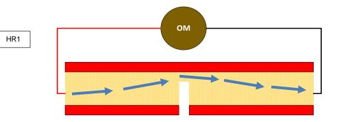
With the circuit fully connected, if you operated the consumer you can see below what would happen to the current flow (in the case of a starter this level of resistance could start a fire due to the excessive heat build-up)
