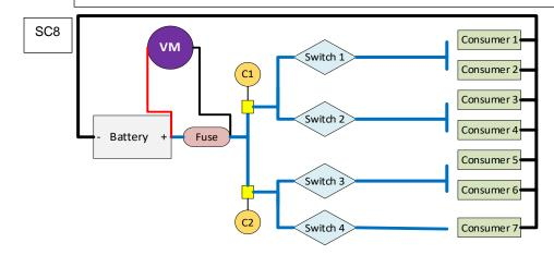
If your reading is battery voltage when a switch is operated then the short is between that switch and the consumer EG "switch 2" below
