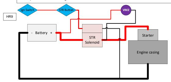
If the reading is now approx 0.5v or less the fault is within the solenoid (don't condemn the solenoid without testing the primary side as a weak pull won't press the switch contacts together properly. You can use the "volt Drop" method on the live from the starter button and test the ground as explained in resistance fault finding) if the reading is higher than approx 0.5v the fault is between the battery and the solenoid.
