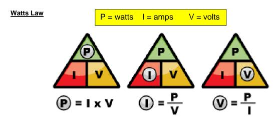
EG: A 60w headlight in a 12v system - 60w/12v = 5 amps
