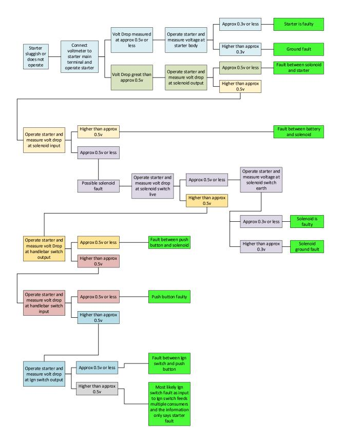
Now that you have diagnosed your electrical fault I will run though some repair methods that should give the best results for a long term "fix" below.
